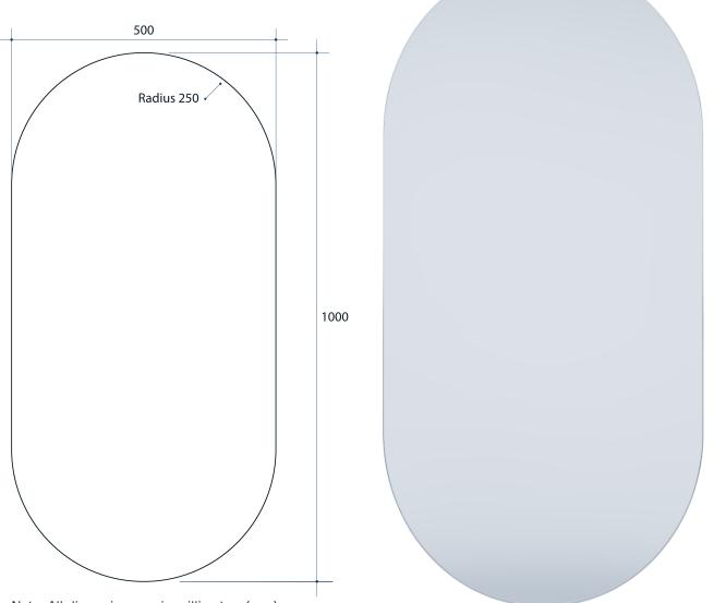
Note: All dimensions are in millimetres (mm)
