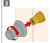
Screw Flange to the Bonnet until flush with wall.
