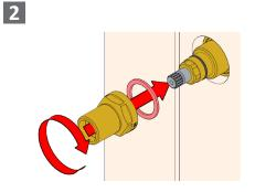
Fit Fibre Washer around the Spindle and then firmly fasten the Bonnet onto the Spindle using a spanner.
