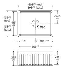
Please note: Butler sink measurements shown are a guide only. For installation, measurements must be taken from physical product received.
